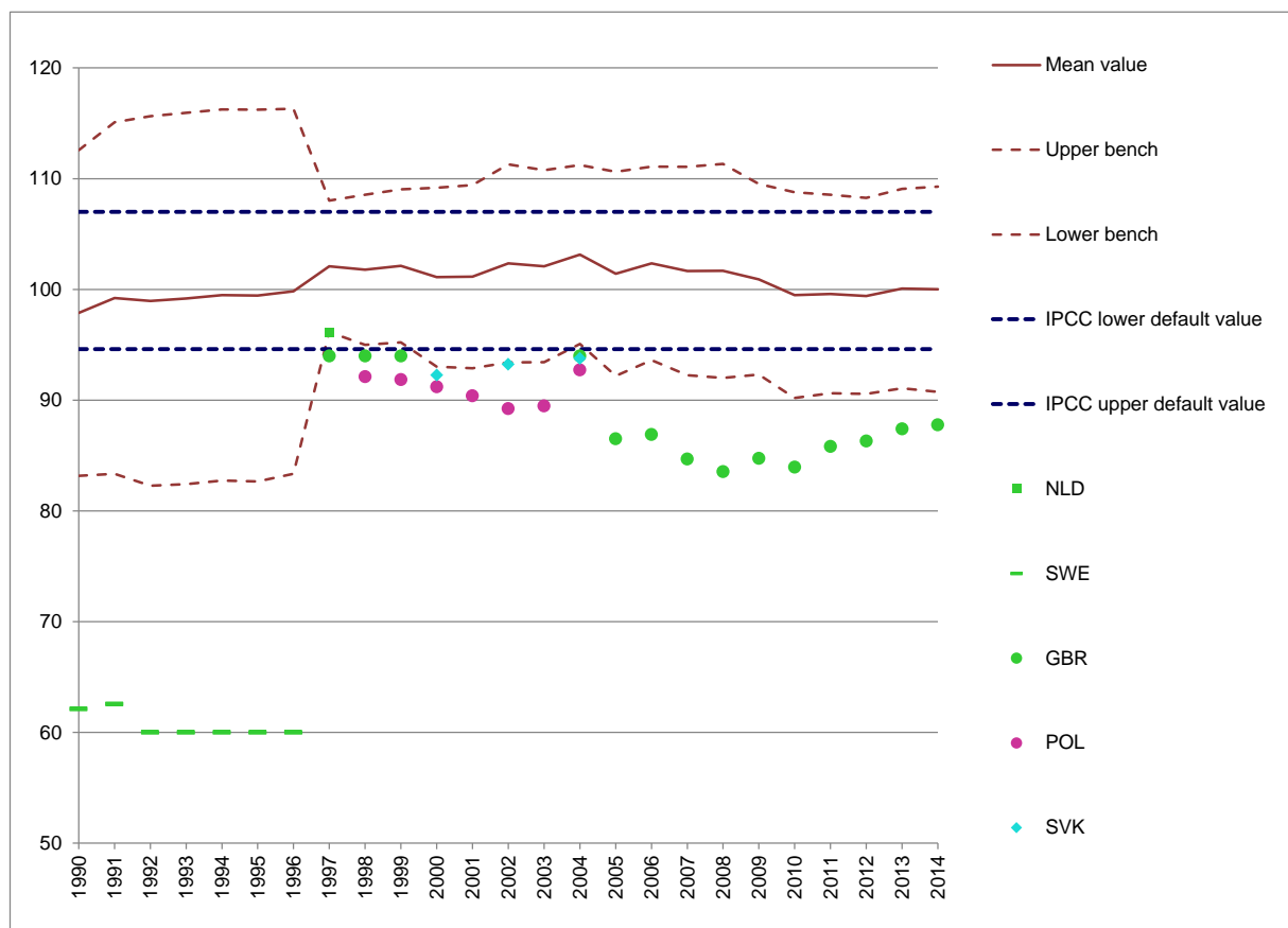
Figure 3.39: 1A2b Non ferrous Metals, solid fuels: Overview of outliers of Implied Emission Factors for CO 2 (in t/TJ)
