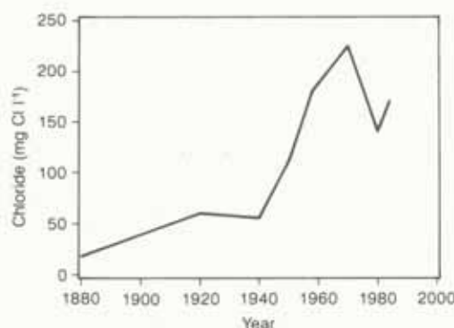
Figure 51: Chloride concentration in the Rhine near Lobith. (Redrawn from van der Weijden & Middelburg, 1989).
