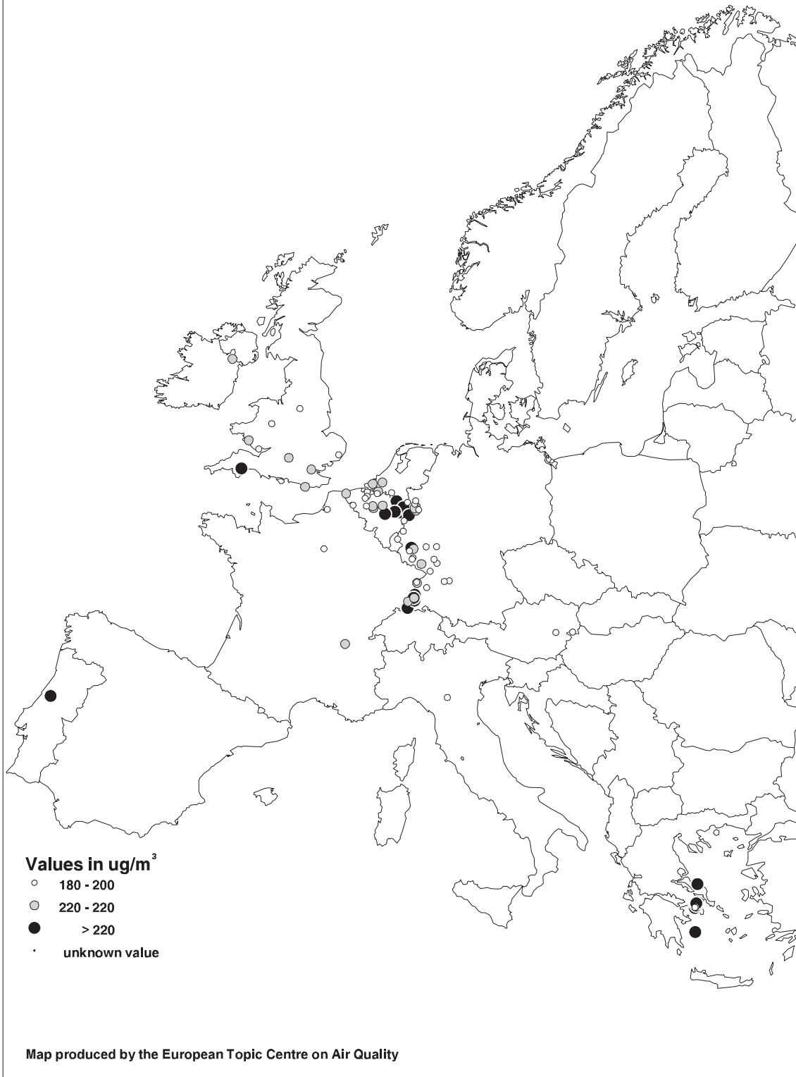
Map 13. Example of an ozone smog episode: hourly ozone concentrations in excess of 180 \mu\text{g}/\text{m}^3 as measured on 1 August 1995.
