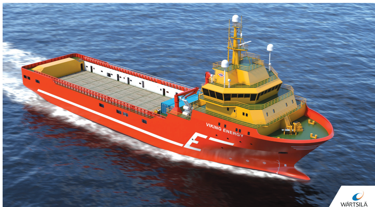
Image A5.5 Viking Energy: the first vessel equipped with a 2MW ammonia powered fuel cell
