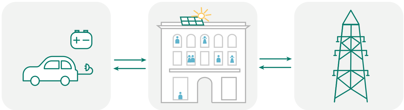
Figure 3.2 Schematic diagram of collective prosumers in one building
